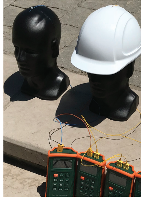
Honeywell tested temperature profiles using hard hats and head forms.
