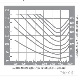
Equivalent sound level contours. Octave band sound pressure levels may be converted to the equivalent A-weighted sound level by plotting them on this graph and noting the A-weighted soundlevel corresponding to the point of highest penetration into the sound level contours. This equivalent A-weighted sound level, which may differ from the actual A-weighted sound level of the noise, is used to determine exposure limits from Table 1.G-16.
