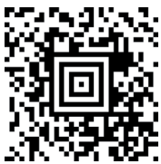
Fig. 4. Aztec Code data is encoded in concentric square rings around the bulls-eye pattern.
